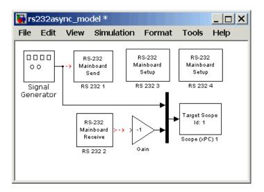
**7** Double-click the first RS-232 Setup block. Enter values to configure the COM1 port on the target PC.
