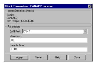
The first dialog entry specifies from which CAN-port the CAN-message should be received.
