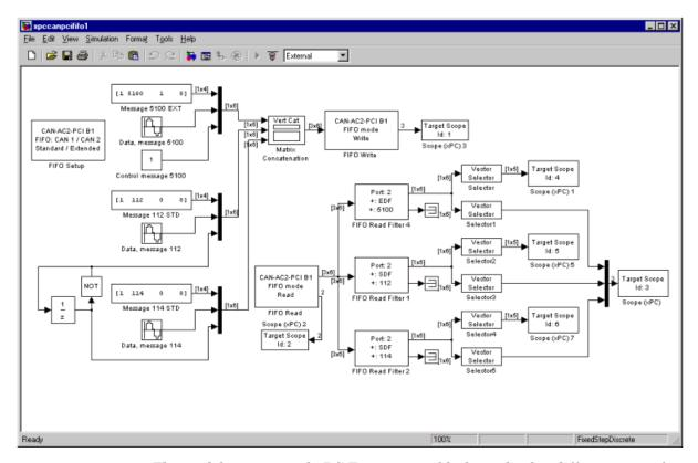
The model uses several xPC Target scope blocks to display different type of data on the target screen:
