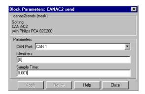
The first dialog entry specifies via which CAN-port the CAN-message should be sent.
