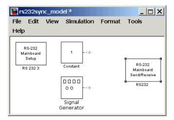
**7** Double-click the RS-232 Setup block. Enter values to configure the COM1 port on the target PC.
