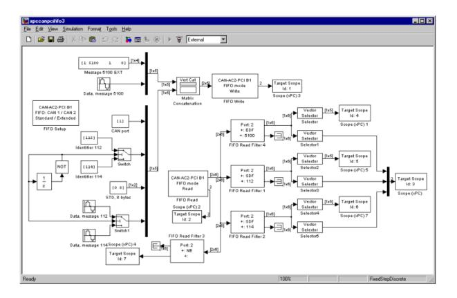
This implementation behaves exactly like the first implementation, but nicely shows how CAN messages (to be sent out) can be constructed dynamically at run-time.
