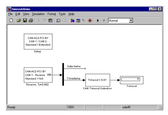
The dialog box of the CAN Time-out Detection block has one edit field and lets you define the time-out value in seconds. The output of the block will be 0 if no time-out has been detected and 1 otherwise. See as well the loop-back example for the CAN-AC2-PCI and CAN-AC2-104 boards (xpccanpci and xpccanpc104) which make use of this utility block as well.
