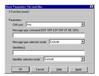
**CAN port** — Defines the filter criterion for the CAN port. From the list, select Any, 1, or 2.
