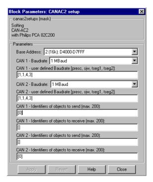
The dialog box allows to define general settings for the CAN-AC2 board. The corresponding code (initializing the board) is executed once during the "initializing blocks" phase after the xPC Target application has been downloaded.
