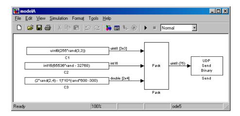
Note that **Port Data Types** and **Signal dimensions** have been turned on from the **Format** menu, showing us that the width of the UDP packet to be sent is 75 bytes. The parameters used in the Pack block are Input port datatypes {'uint8', 'int16', 'double'} and Byte Alignment 1.
