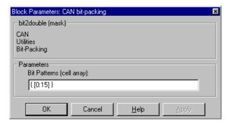
The dialog box contains one single control (edit field) which lets you define the bit patterns in a flexible way. The data type entered in the control has to be a MATLAB cell array vector. The number of elements in the cell array define the number of input ports shown by this block instance. The cell array elements have to be of type double array and define where each bit of the incoming value (data typed input port) comes to lie at what position in the outgoing double value (data frame).
