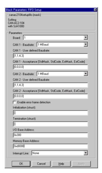
**Board** — Define which board is being accessed by this driver block instance. If multiple boards are present in the target system, the board number (1, 2 or 3) can be seen as a reference identifier in order to differentiate the boards. The physical board finally referenced by the board number depends on the PCI Slot
