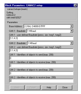
The dialog box allows you to define general settings for the CAN-AC2 board. The corresponding code (initializing the board) is executed once during the "initializing blocks" phase after the xPC Target application has been downloaded.
