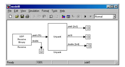
For setting up the Receive block, **IP address to receive from** is set to 192.168.0.1 (the hypothetical address of the system that will run Model B). The **IP port to receive from** is set to 25000 (the same value as set in the Send block in Model A). The **Output port width** is set to 75 which is obtained from the output port width of the Pack block in Model A.
