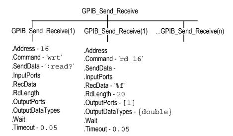
Currently, only two limitations exist. xPC Target does not support string data types as input and output data types. Also, you must know the size and order of data returned from a read command.
