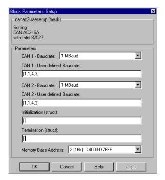
**CAN 1 - Baud rate** — The first control (pop-up menu) lets you define the most common baud rates for CAN port 1. If special timing is necessary (baud rate), the value "User defined" can be selected. In this case the second control (edit field) is used to provide the four values for the timing information. The vector elements have the following meaning:
