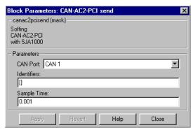
The first dialog entry specifies via which CAN-port the CAN-message should be sent.
