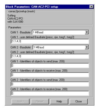
The dialog box allows to define general settings for the CAN-AC2-PCI board. The corresponding code (initializing the board) is executed once during the "initializing blocks" phase after the xPC Target application has been downloaded.
