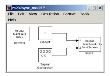
8 Set the PreLoadFon for your Simulink model to load the message structures when you open your model. For example, if you saved the message structures in the M-file RS232Sync messages, type
