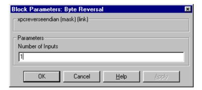
This block takes just one parameter, the number of inputs. The number of input ports adjusts automatically to follow this parameter, and the number of outputs is equal to the number of inputs.
