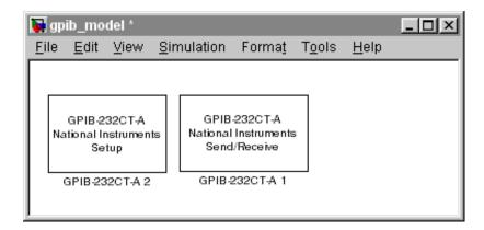
5 Double-click the GPIB Setup block. Enter values that correspond to the DIP switch settings you set on the GPIB-232CT-A controller. In the **Initialization Struct** box, enter the name for the MATLAB structure this block uses to send initialization messages to the GPIB device.
