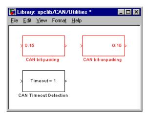
The main purpose of the two blocks is to be used in conjunction with CAN Send and Receive driver blocks, but they can be used as well for other types of data manipulation. Their functionality is entirely independent of any CAN driver blocks or CAN library.
