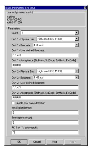
**Board** — Defines which board is being accessed by this driver block instance. The board number (1...3) can be seen as a reference identifier in order to differentiate the boards if multiple boards are present in the target system. The physical board finally referenced by the board number depends on the PCI
