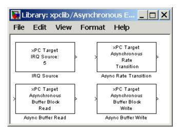
**3** Drag-and-drop the xPC Target IRQ block in your Simulink model and connect the output to this block to the input of a Function-Call Subsystem. For more information on Function-Call subsystems, see *Using Simulink* and the *Real-Time Workshop User's Guide*.
