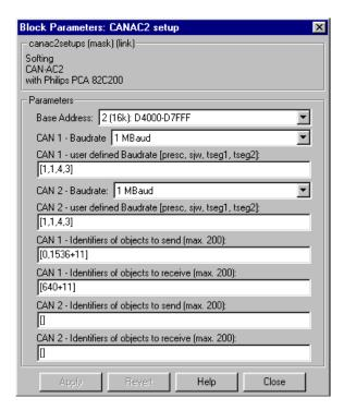
The Receive block receives the data (PDO) over CAN-message 640+node-i and must look as follows:
