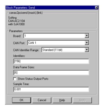
The data frame is then propagated to the CAN Send driver block and is sent out as part of a CAN-message having identifier 156. When looking at the Send block's dialog box, the data frame size is defined as 6 bytes. This makes sure that only the first 6 bytes of the incoming double value are transmitted as part of the CAN-message.
