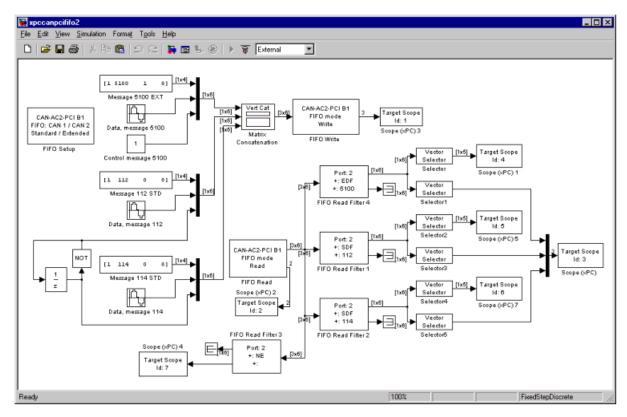
Having observed this, we could then reduce the Read depth of the FIFO Read block from 3 to 2. This would not change anything of the overall behavior of the model. As a positive side effect, the latency time of the FIFO Read block gets smaller and therefore the model's cycle time as well.
