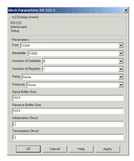
For more information on entering the block parameters, see "RS-232 Setup Block" on page 1-27. For the procedure to create the initialization and termination structures, see "RS-232 MATLAB Structure Reference" on page 1-32.
