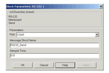
For information on entering the block parameters, see "RS-232 Send Block (Asynchronous)" on page 1-30. For the procedure to create the send structure, see "RS-232 MATLAB Structure Reference" on page 1-32.
