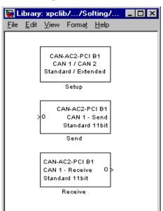
The third block group highlighted above contains the three available CAN blocks: Setup, Send, and Receive.
