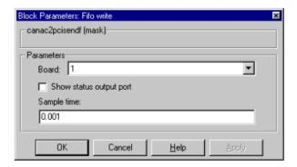
**Board** — Define which physically present board is used to send out the CAN messages defined by this block instance. For more information about the meaning of the board number see the Setup driver block described above. If just one board is present in the target system, you should select 1.
