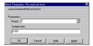
**Board** — Defines which physically present board is accessed to read the current transmit FIFO level. For more information about the meaning of the board number see the Setup driver block described above. If just one board is present in the target system, board number 1 should be selected.
