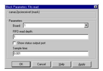
**Board** — Defines which physically present board is used to send out the CAN messages defined by this block instance. For more information about the meaning of the board number see the Setup driver block described above. If one board is present in the target system, select board number 1.
