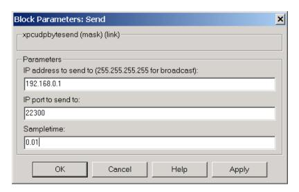
The **IP** address to send to and the **IP** port to send to have to be specified in the appropriate locations. The local IP port that is used for sending will be determined automatically by the networking stack. The sample time should be set to an appropriate value, with similar considerations as in the receive block.
