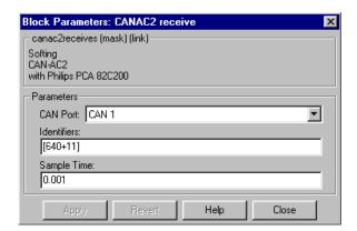
If more than one CANopen device is connected to the network, the dialog boxes of the Setup and Receive blocks and the CANAC2\_setup.c file have to be extended accordingly. If you need for-loops in the CANAC2\_setup.c, use the variable CANAC2\_counter.
