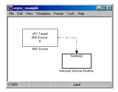
In the setup shown above, the CPU executes the contents of the Function Call-Subsystem whenever IRQ 5 occurs.
