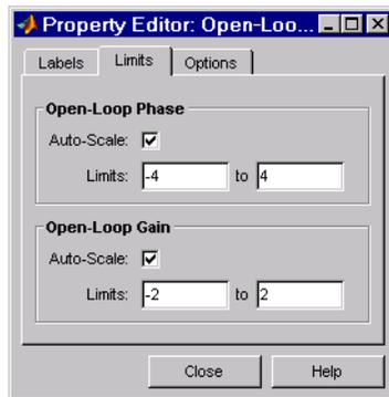
To change the limits, specify the new values in the **Limits** fields for open-loop phase and/or gain. The **Auto-Scale** check box automatically deactivates once you click in a different field. The Nichols plot updates immediately.
