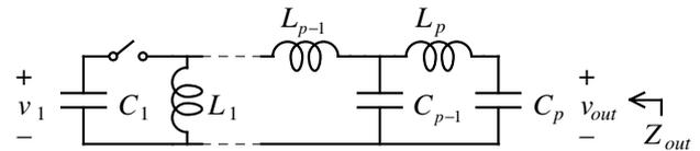
Figure 1. Low-pass transformerless multiple resonance network.
