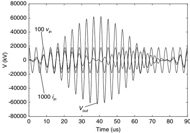
Figure 5. Voltages and input current for cosinusoidal input.
