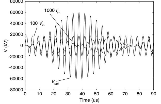
Figure 7. Voltages and input current for sinusoidal input.
