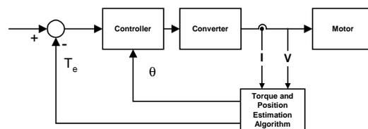
Figure 5 – Estimation and control of a SR Motor
