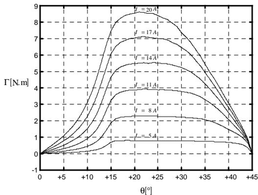
Figure 3 - Phase Torque -  $\Gamma(\theta, I)$ .
