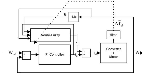
Figure 10 – Simplified diagram with the PI controller and “neuro-fuzzy” compensator
