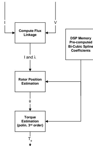
Figure 4 – Position and torque estimation
