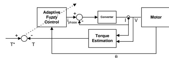
Figure 9 – Fuzzy adaptive control for torque ripple in SR motor
