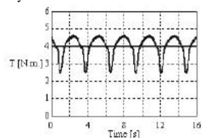
Fig. 1. Torque ripple from constant current reference.
