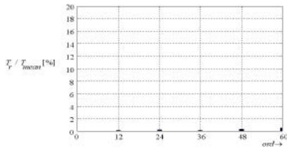
Fig. 13. Harmonic content in torque signal.
