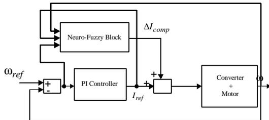
Fig. 3. PI control and the neuro-fuzzy compensator.
