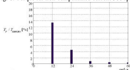
Fig. 9. Harmonics of non-compensated torque. After one training iteration, the torque harmonic content is already significantly lower, as shown in Figures 10 and 11. The 12th harmonic has a relative magnitude of only 3% approximately.
