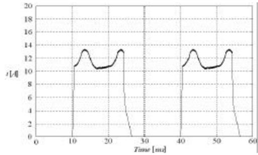
Fig. 14. Current pulses after 10 iterations.
