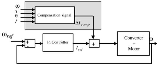
Fig. 2. SR drive with the compensating signal.
