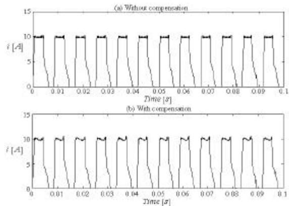
Fig. 15. Phase current A – 1800 rpm.
