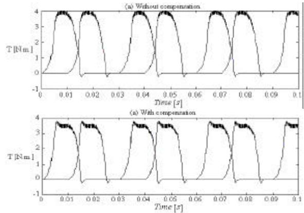
Fig. 20. Torque in phases A and B – 500 rpm.
