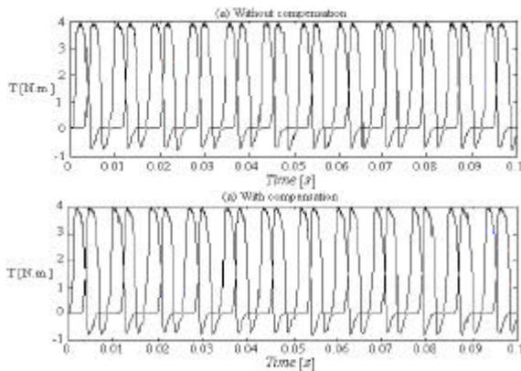
Fig. 19. Torque in phases A and B – 1000 rpm.
