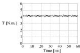
Fig. 12. Compensated torque after 10 iterations.
