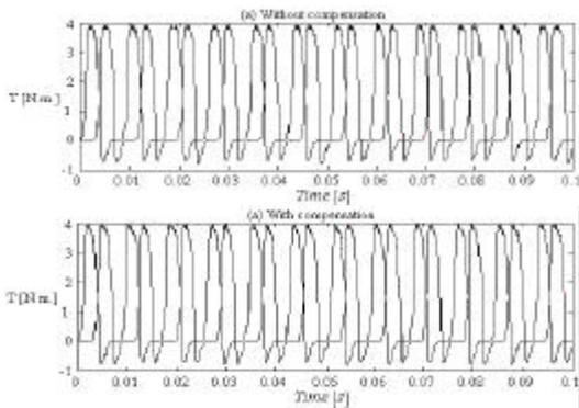
Fig. 18. Torque in phases A and B – 1800 rpm.
