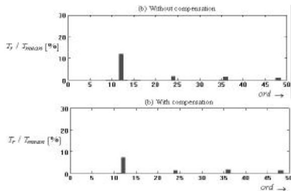
Fig. 25. Torque frequency spectrum – 1000 rpm.
