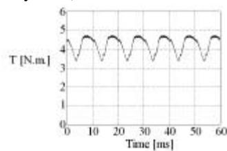
Fig. 8. Torque for non-compensated current 500 rpm.
