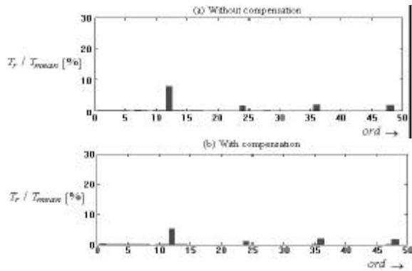
Fig. 24. Torque frequency spectrum – 1800 rpm.
