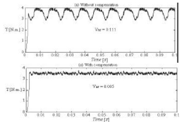
Fig. 23. Total torque – 500 rpm.
