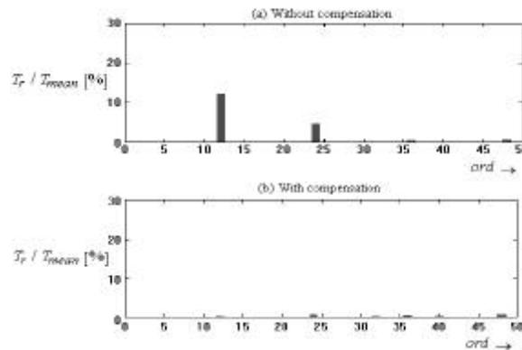
Fig. 26. Torque frequency spectrum – 500 rpm.
