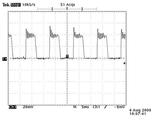
Fig. 12. Currents regulated by the hysteresis controller. (Vert.: 1A/div and Hor.: 25ms/div  $\cong$  20 mech. degrees)
