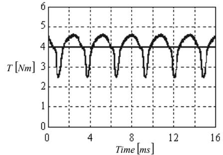
Fig. 5. Simulated result showing the torque ripple from a constant current reference.
