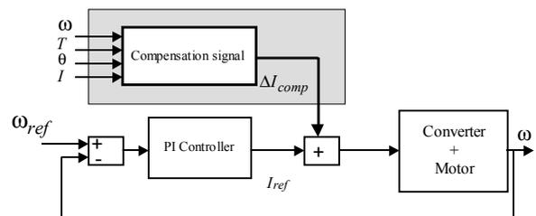
Fig. 6. SR drive with the compensating signal.
