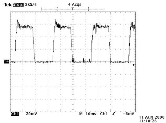
**Fig. 19. PI cont. + external load (no compensation). (Vert.: 1A/div and Hor.: 50ms/div  $\cong$  40 mech. degrees)**
