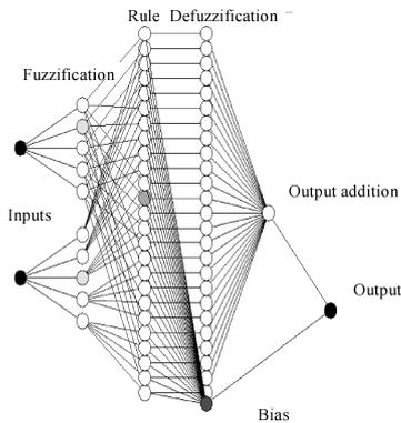
Fig. 7. Neuro-fuzzy structure of the compensator.
