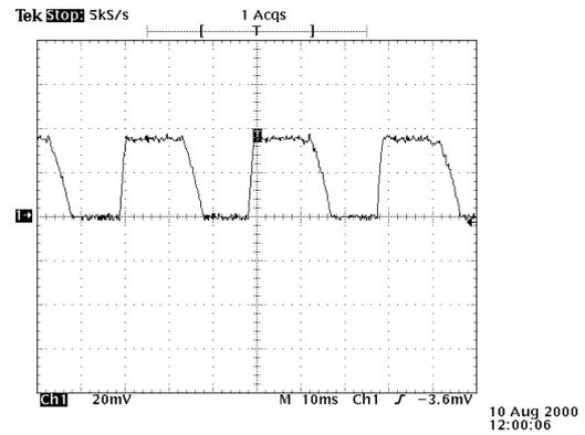
Fig. 13. Phase current without compensation. (Vert.: 1A/div and Hor.: 50ms/div  $\cong$  40 mech. degrees)
