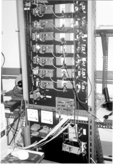
Fig. 11. H-bridge power converter.
