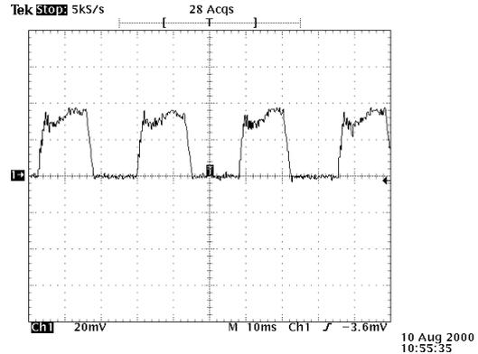
Fig. 14. Phase current with compensation. (Vert.: 1A/div and Hor.: 50ms/div  $\cong$  40 mech. degrees)
