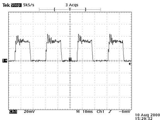
**Fig. 17. PI closed-loop without compensation. (Vert.: 1A/div and Hor.: 50ms/div  $\cong$  40 mech. degrees)**
