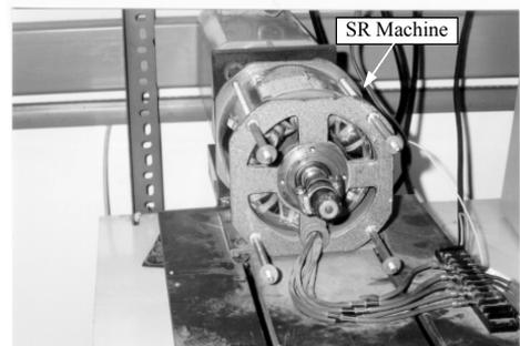
Fig. 10. Stator and rotor elements of the 6/4 SR machine.
