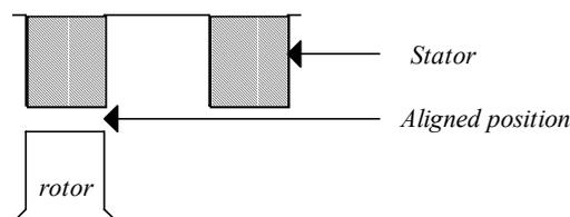
Fig. 1. Aligned position.
