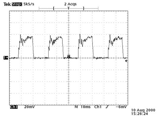
**Fig. 18. PI closed-loop with compensation. (Vert.: 1A/div and Hor.: 50ms/div  $\cong$  40 mech. degrees)**
