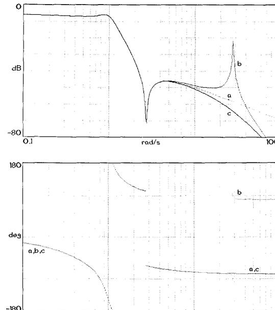
Fig. 2 - Frequency responses obtained for the OTA-C filter in fig. 1. (a) With ideal OTAs and no parasitic capacitances. (b) Considering the parasitic capacitor  $C_p$ . (c) Reversing the polarities of the marked OTAs.
