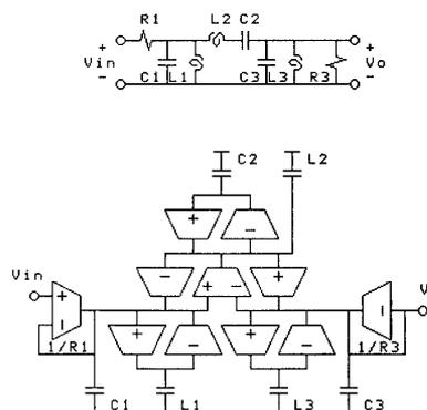
Fig. 3 - OTA-C simulation for a passive all-pole band-pass filter.
