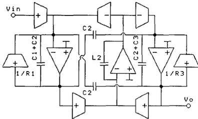
Fig. 5 - OTA-C-0A simulation for the 3th order elliptic low-pass filter shown in fig. 1.
