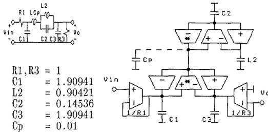
Fig. 1 - Normalized OTA-C filter simulation for an elliptic low-pass filter (left) with 1 dB passband ripple from 0 to 1 rad/s and 40 dB minimum attenuation at the stopband. A small parasitic capacitor,  $C_p$ , is considered connected as shown, being equivalent to the parasitic inductor  $L_c$  shown in the prototype filter. In this and in the other drawings, the transconductances are unitary unless when otherwise indicated.
