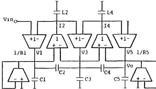
Fig. 6. Economical OTA-C simulation of the filter in fig. 4.
