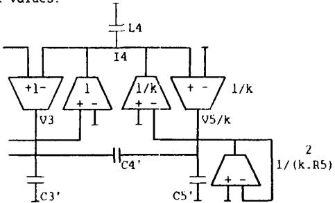
Fig. 7. Voltage level scaling in the circuit in fig. 6.  $V_5$  is changed to  $V_5/k$  without any change in other voltages.  $C_3' = C_3 + (1-k) \cdot C_4$ ,  $C_4' = k \cdot C_4$ , and  $C_5'' = k \cdot (k \cdot C_5 + (k-1) \cdot C_4)$ .
