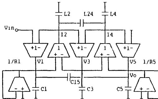
Fig. 9. OTA-C simulation of the circuit in fig. 8.
