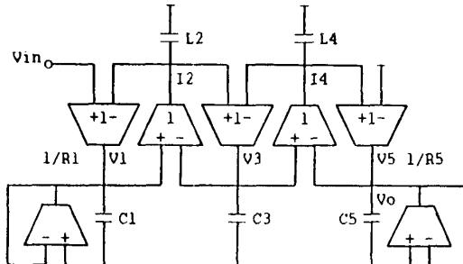
Fig. 2. OTA-C "leapfrog" realization of the filter in fig. 1.
