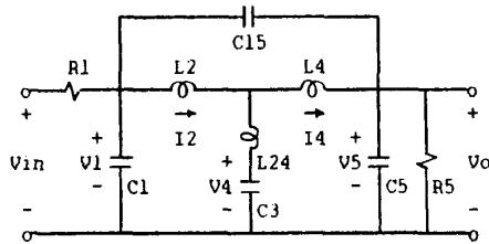
Fig. 8. Unbalanced lattice realization for a 5th-order low-pass filter with finite transmission zeros.
