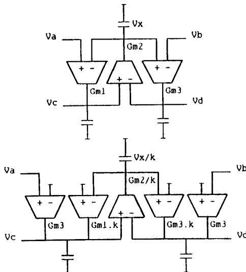
Fig. 3b. Changing  $V_x$  to  $V_x/k$  without changing  $V_a, \dots, V_d$ .
