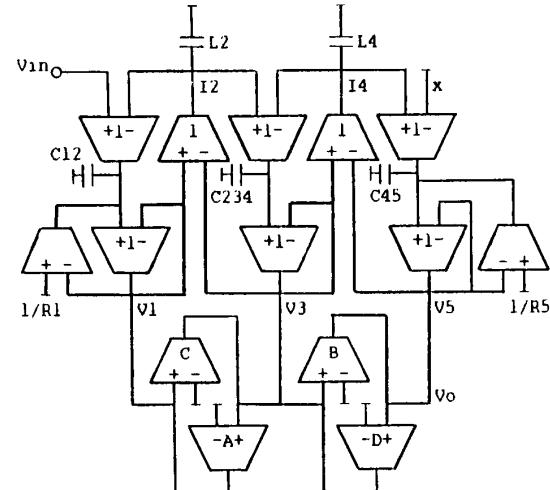
Fig. 5. Normalized OTA-C simulation of the filter in fig. 4. Version with OTAs coupling the states.  $C12 = C1+C2$ ,  $C234 = C2+C3+C4$ ,  $C45 = C4+C5$ ,  $A = C2/(C1+C2)$ ,  $B = C4/(C4+C5)$ ,  $C = C2/(C2+C3+C4)$  and  $D = C4/(C2+C3+C4)$ .
