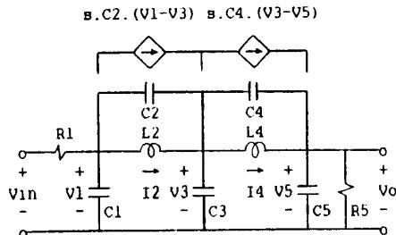
Fig. 4. Mid-series ladder with bridging capacitors replaced by controlled sources.
