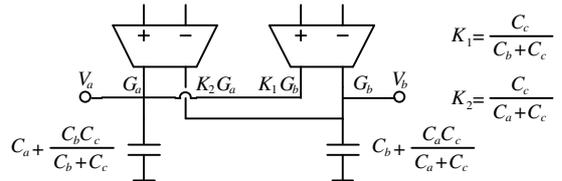
Fig. 6. Implementation of the current-controlled Norton equivalent for a capacitor loop.
