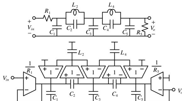
Fig. 1. Passive prototype and normalized OTA-C structure with multiple capacitor loops for a 5th-order elliptic low-pass filter.
