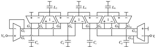
Fig. 8. Normalized OTA-C simulation of the structure in fig. 7c (with  $R_1=R_7=1$ ), with the capacitor loops eliminated.
