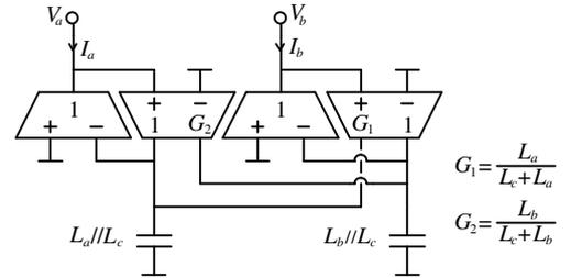
Fig. 11. OTA-C implementation of the voltage-controlled Thévenin equivalent for a simple inductor loop.
