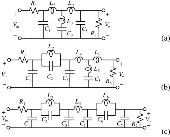
Fig. 7. Some LC doubly terminated structures for low-pass filters with separated capacitor loops or inductor cut-sets. (a) 5th-order with only 2 finite transmission zeros (the normal is 4). (b) 6th-order with 4 finite transmission zeros (the maximum possible for LC doubly terminated realization). (c) 7th-order with only 4 finite transmission zeros (the normal is 6).
