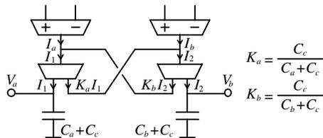
Fig. 4. Schematic representation of an implementation of the voltage-controlled Norton equivalent of a capacitor loop.
