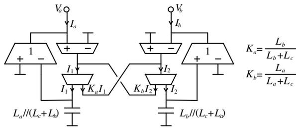
Fig. 13. Schematic representation of the OTA-C realization of the current-controlled Thévenin equivalent for an inductor loop.
