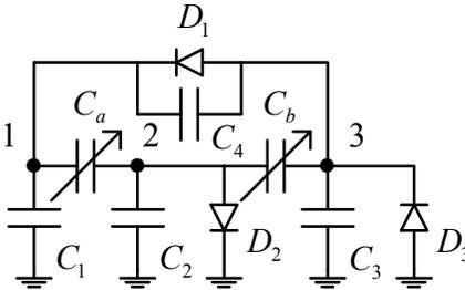
Figure 4. Bennet's doubler with diodes instead of contact switches.
