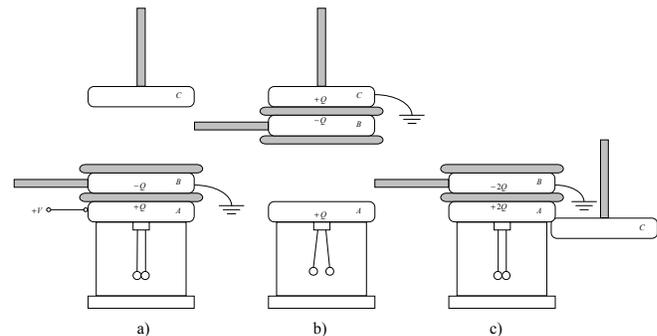
Figure 2. Bennet's doubler connected to an electroscopes.
