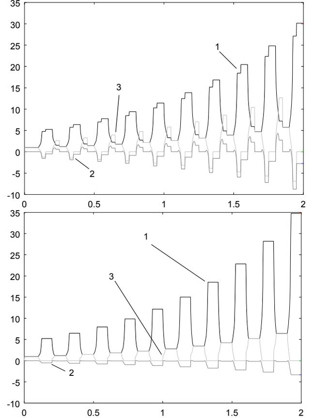
Figure 5. Simulations of the doublers with switches (above) and with ideal diodes (below), showing the three nodal voltages along the time.
