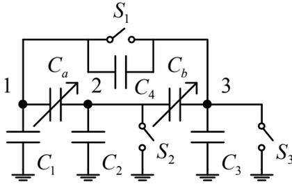
Figure 3. "Switched capacitor" model of Bennet's doubler.
