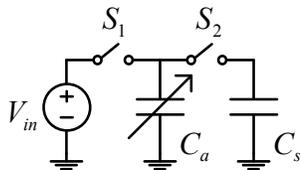
Figure 1. Basic electrostatic energy harvester.
