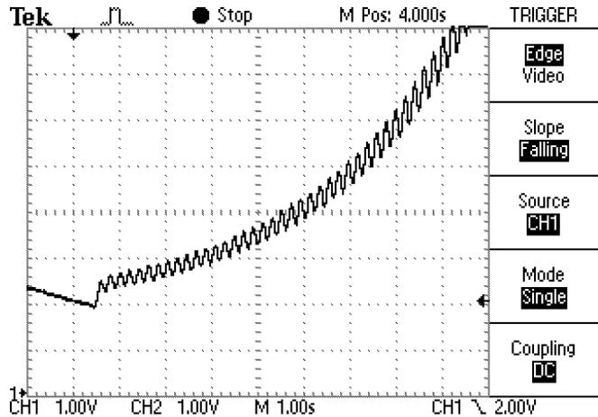
Figure 7. Measurement of the charging waveform at  $C_1$ . 100 V/div.
