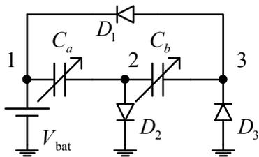
Figure 6. Simple battery charger.
