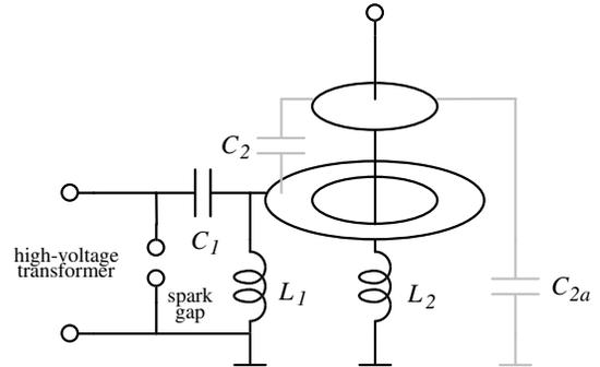
**Figure 5.** 4<sup>th</sup>-order experimental circuit with distributed capacitances  $C_2$  and  $C_{2a}$ .
