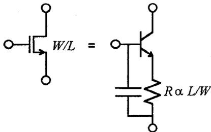
Fig. 1. Basic bipolar equivalent of a MOS transistor.
