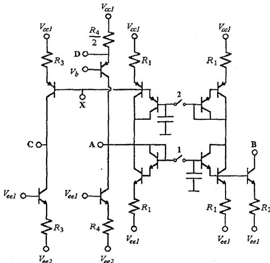
Fig. 3. First-generation integrator, with inverting ("B") and noninverting ("C") outputs, and two possible equivalent inputs ("A", "D"). Point "X" is used in the output circuit (fig. 4).
