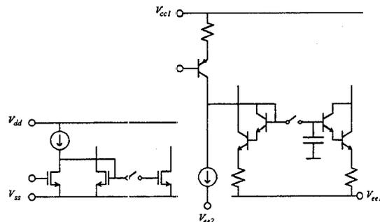
Fig. 2. Example of conversion from a CMOS SI "first generation" structure, showing the necessary changes.
