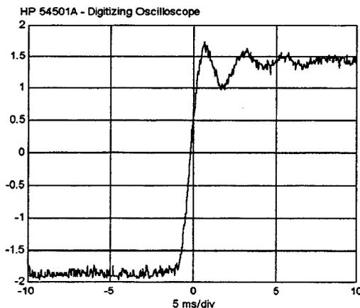
Fig. 5. Transient response of a step transition, used to evaluate the filter performance.
