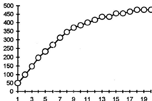
Fig. 7. Measured oscillating frequency of the transient response (Hz) versus switching frequency (kHz) in the test filter.
