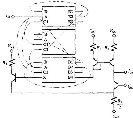
Fig. 4. Interconnection of 3 integrators, building a 3rd-order bilinear elliptic filter.
