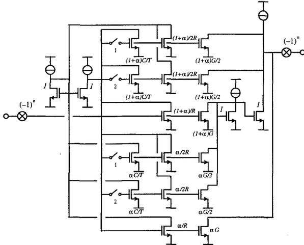
**Fig. 4.** Lossy bilinear integrator with clock feedthrough compensation by scaled replica.
