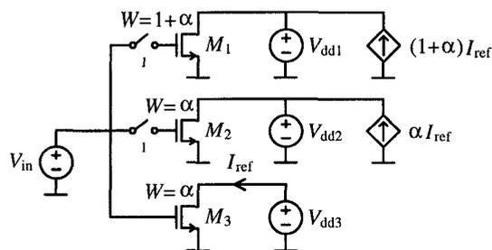
Fig. 5. Model used in the evaluation of the current replication technique.
