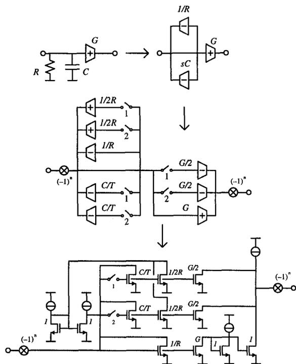
Fig. 3. "Modulated" component-simulation implementation of a lossy bilinear integrator.
