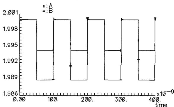
Fig. 6. Gate voltages for  $M_1$  (A) and  $M_2$  (B).
