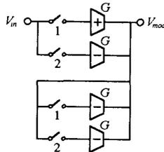
Fig. 11. Modulator circuit, that operates with a two-phases non-overlapping clock.
