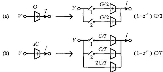
Fig. 2. Bilinear "transconductor" (a) and bilinear "transcapacitor" (b).
