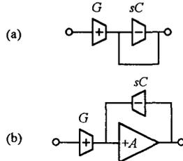
Fig. 5. Integrators: Transconductor-C (a) and Miller (b)
