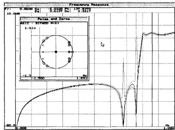
Fig. 8. High-pass filter obtained by the "reverse mapping" of the prototype. The gain frequency response is shown, with expected error margins, and again the poles and zeros. Note the transformation  $H(z) \rightarrow H(-z)$ .
