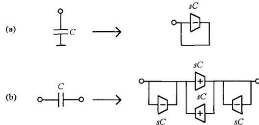
Fig. 4. Grounded capacitor and floating capacitor construction using transcapacitances.
