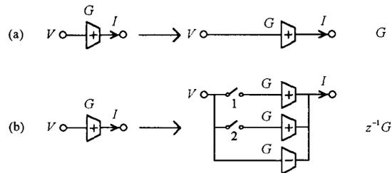
Fig. 3. Backward Euler (a) and forward Euler (b) "transconductors".
