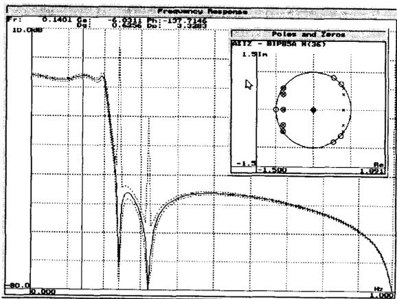
Fig. 10. Low-pass filter gain, error margins, and poles and zeros, obtained by the "modulation" of the input and output signals of the "reverse mapped" example filter.
