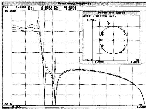
Fig. 7. Gain frequency response of a "normal" bilinear SI low-pass filter, with expected error margins and poles and zeros in  $z^{1/2}$ .
