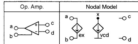
Fig. 3. Ideal operational amplifier, and its nodal model.
