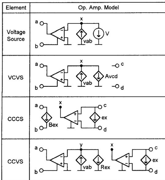
Fig. 4. Models for the special elements using ideal op.amps.
