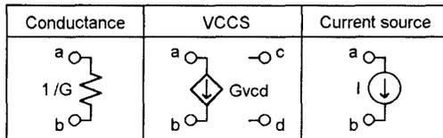
Fig. 1. Circuit elements allowed in the basic nodal analysis method.
