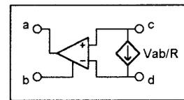
Fig. 5. Alternative simpler model for the CCVS, when  $R \neq 0$ .
