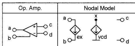
Fig. 3. Ideal operational amplifier, and its nodal model.
