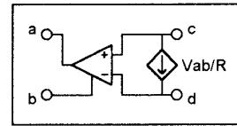
Fig. 5. Alternative simpler model for the CCVS, when  $R \neq 0$ .
