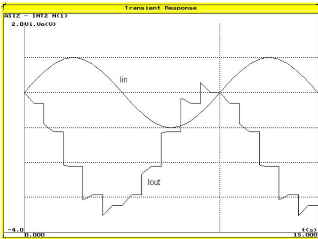
Fig. 3. Transient response  $I_{out}$  for a 0.1 Hz, 1 A, sinusoidal input  $I_{in}$ . Above: S/H input. Below: Continuous input.
