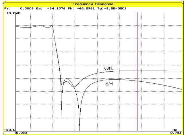
Fig. 7. Effect of direct signal feedthrough in the filter in fig. 6.
