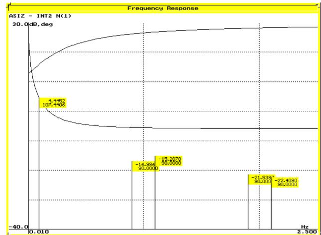
Fig 5. Frequency responses, now in linear frequency scale, with the first spectral components plotted, for a 0.1 Hz cosinusoidal input. Above: S/H signals. Below: continuous signals.
