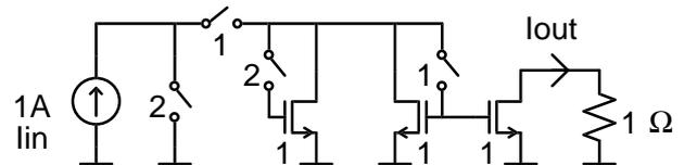
Fig. 2. Normalized “second generation” SI integrator, used as example of direct signal feedthrough and spectrum calculations.
