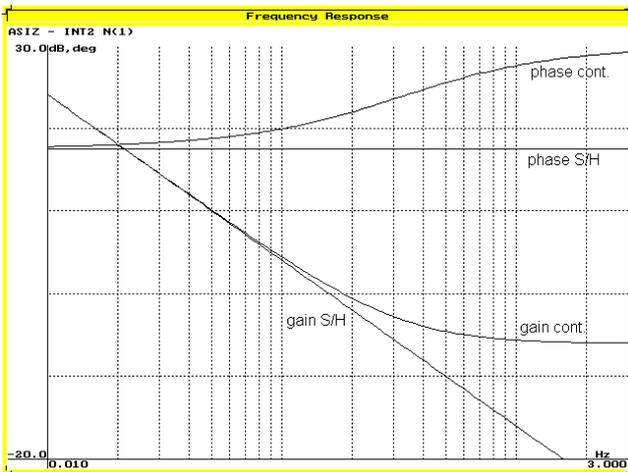
Fig. 4. Frequency responses (gain and phase) for the SI integrator, considering the input sampled and held and considering it continuous.
