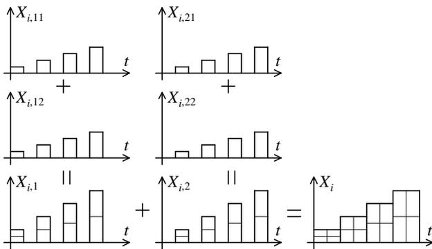
Fig. 1. Composition of signals in a two-phases SI or SC circuit.
