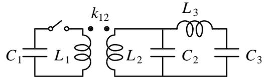
Fig. 2. Triple resonance network with a transformer and additional inductor and capacitor.
