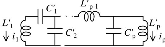
Fig. 5. multiple resonance network for energy transfer between inductors.  $L'_1 = \alpha C_1$ ,  $C'_2 = L_2/\alpha$ , etc.
