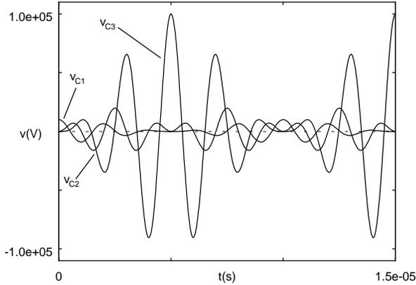
**Fig. 3. Typical triple resonance network, and voltages in  $C_1$ ,  $C_2$ , and  $C_3$  after the closure of the switch.  $C_1=1$  nF,  $C_2=126.3$  pF,  $C_3=10$  pF,  $L_1=110$   $\mu$ H,  $L_2=780.7$   $\mu$ H,  $L_3=10.13$  mH,  $k_{12}=0.28131$ .**
