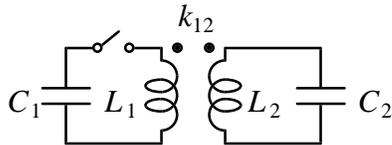
Fig. 1. Double resonance network with a transformer.
