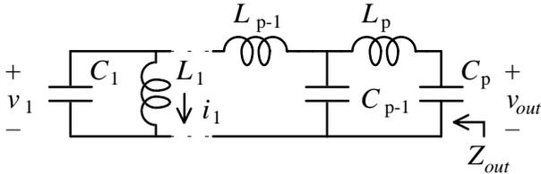
**Fig. 4. Transformerless multiple resonance network.**
