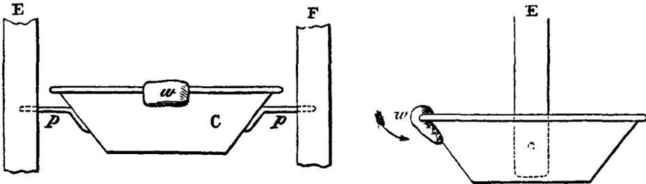
the receivers are nearly full of water, their balance is such that they turn in the opposite direction and so empty themselves. The four receivers are made to turn towards the axis of the machine and to deliver the water into a metal bath, which for continuous action should be connected with a drain.
