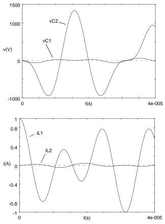
Fig. 6. Energy transfer between  $L_1$  and  $C_2$  in a double resonance network with a transformer.
