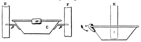
the receivers are nearly full of water, their balance is such that they turn in the opposite direction and so empty themselves. The four receivers are made to turn towards the axis of the machine and to deliver the water into a metal bath, which for continuous action should be connected with a drain.
